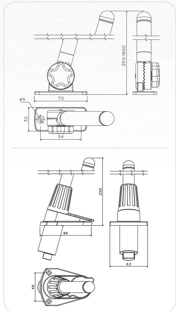
**Installation:** Should be screwed in such a position in order to be higher than the sidelights (according to COLREG 72)
